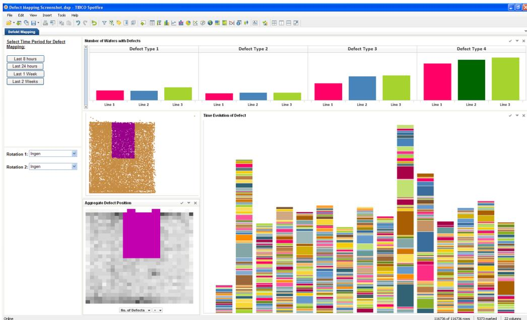
Spotfire's heat map visualization is used to identify the wafer position with the most defects. Drill down capability enables users to find out when the problem causing the defects began.
